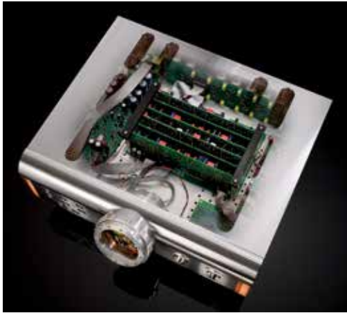
There are 6 vertically mounted daughter boards, one for each input.
