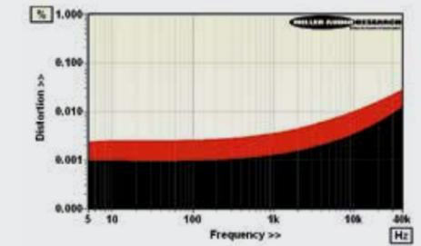
**ABOVE:** Distortion versus extended frequency (1W/8ohm, black; 100W/8ohm, red)
