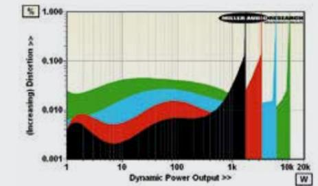
**ABOVE:** Dynamic power output versus distortion into 8ohm (black trace), 4ohm (red), 2ohm (blue) and 1ohm (green) speaker loads. Max. current is 106A (!)
